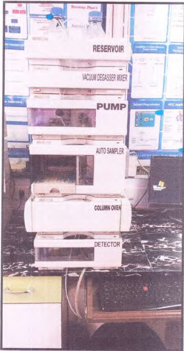
Reservoir, Vacuum Degasser Mixer, Pump, Auto Sampler, Column oven, Detector
