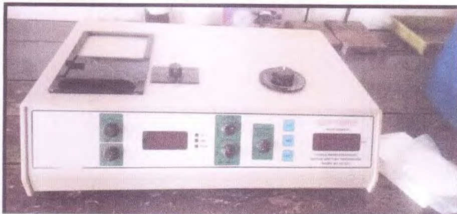
Spectro photo meter for detection of N and P
