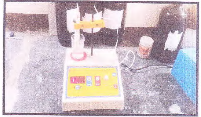
pH Meter for detection of Acidic and Basic soil and water
