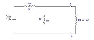
12. Using Norton's theorem find out the current passing through load resistance RL.
