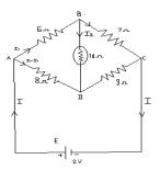
15. Obtain the Thevenin's and Norton's equivalent circuits of the network given below.
